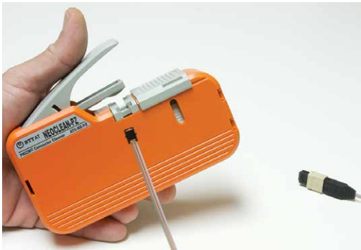
Placing PRIZM® LightTurn® connector into cleaner
