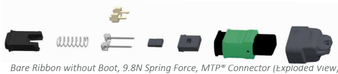
Bare Ribbon without Boot, 9.8N Spring Force, MTP® Connector (Exploded View)
