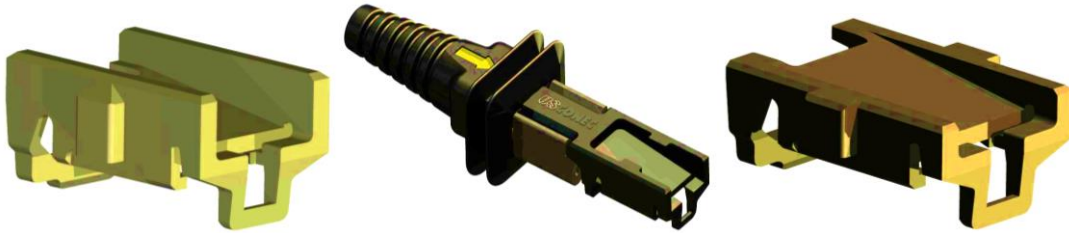
Figure 5. 5a) The standard connector housing protects the lens array while providing latching features to connect to the VCSEL interface. 5b) Round cable version of the housing provides improved strain relief while adding an outer housing to help seal the VCSEL module against outside contamination. 5c) Reduced height connector housing for low-overhead applications.
