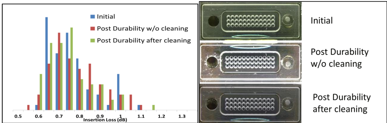
Figure 2: Insertion Loss Histogram for Initial, Post Durability without cleaning, and after a cleaning iteration.
