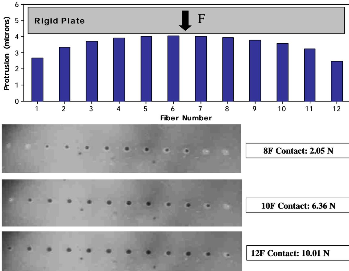
Figure 11: Sample tip deflection vs. reaction force data
