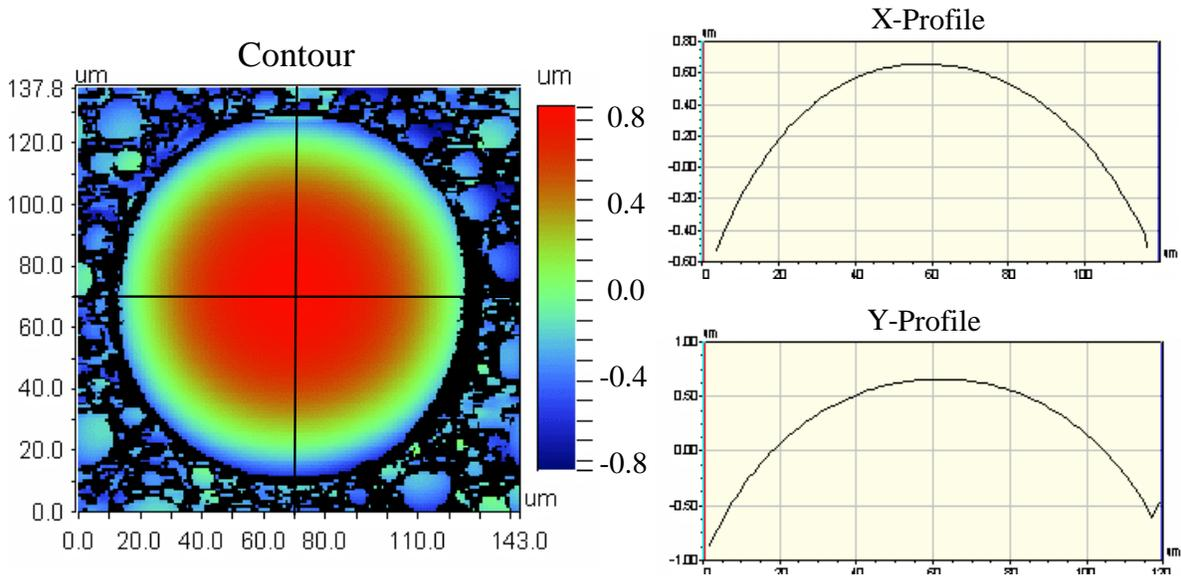
Figure 9: Typical interferometric endface analysis of fiber tip
