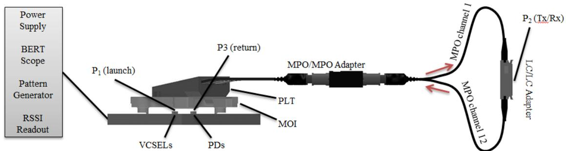
Figure 9. Schematic for empirical testing of insertion loss of MOI and associated link.  $P_1$  indicates the reference power exiting the VCSEL,  $P_2$  is the power measured via wide-area detector, and  $P_3$  is the power measured on return by the PD.
