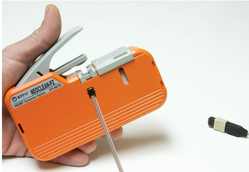
Placing PRIZM® LightTurn® connector into cleaner
