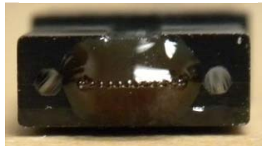
Image 2 Not recommended bead size
