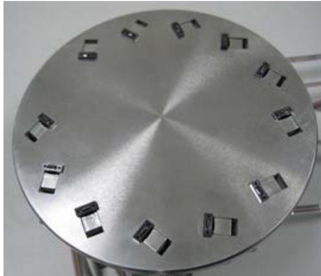
Image 7 Consistent bead size throughout fixture
