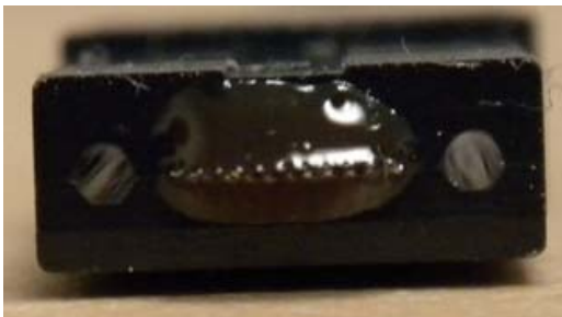
Image 1 Recommended bead size
