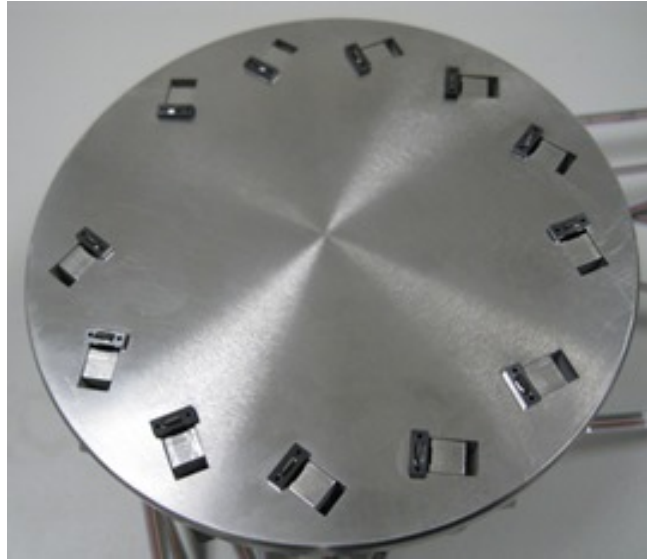
Image 7 Consistent bead size throughout fixture
