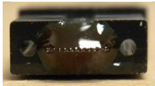
Image 2 Not recommended bead size
