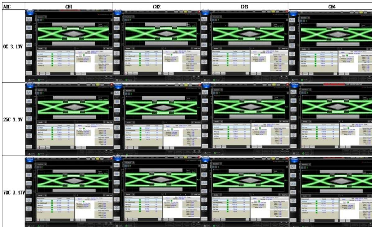
Figure 16. A four channel AOC running at 25 Gbps using the MOI and PLT connector for coupling. The AOC was cycled from 0°C to 70°C (rows 1 to 3, respectively) and showed no degradation in performance.
