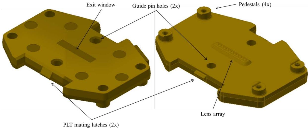
Figure 1. The MOI major features: (left) top side of the MOI, where the PLT ferrule mates using alignment guide pins and (right) bottom side of the MOI, where the lens array is aligned to the VCSEL/PD to capture and couple light.
