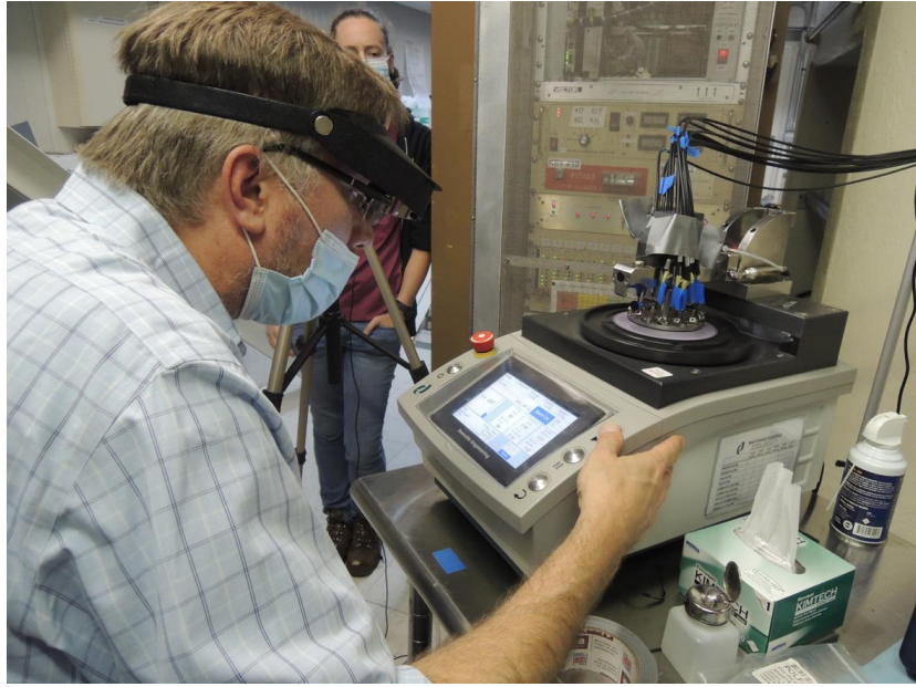
Figure 9: A set of 12 MTP ferrules are polished with the automated polishing machine.
