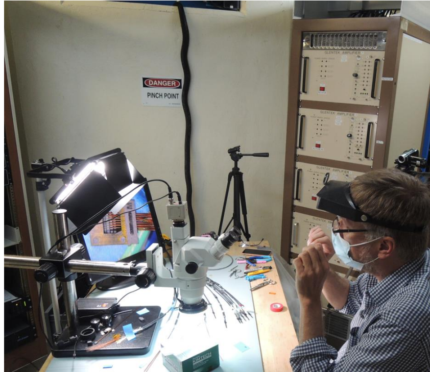
Figure 7: Installing fibers within ferrules with the aid of a high-magnification digital microscope. The pigtail of fibers that normally extends up to the telescope and terminates in the male gang connector has been retracted and is seen draped against the wall that surrounds the cone bearing supporting the telescope so the connectors can be replaced on the workbench.
