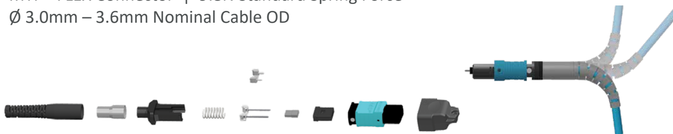
Round, 9.8N Spring Force, MTP® FLEX Connector (Exploded View)
