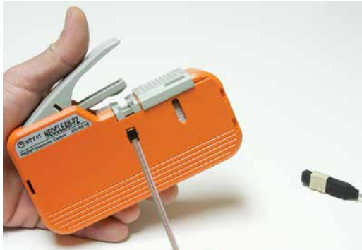
Placing PRIZM® LightTurn® connector into cleaner
